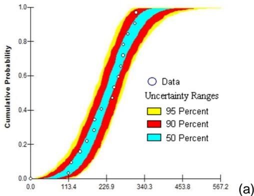
Figure 3 Probability band of  $SO_2$  EFs for “1A1a-10101-3.10” as cumulative distribution of Weibull distribution fitted to  $SO_2$  EFs derived from in-situ measurements
